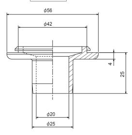
The outdoor unit is provided with several holes for drainage at the bottom to ma easier. The drain socket is used to close the unnecessary holes and centralize
