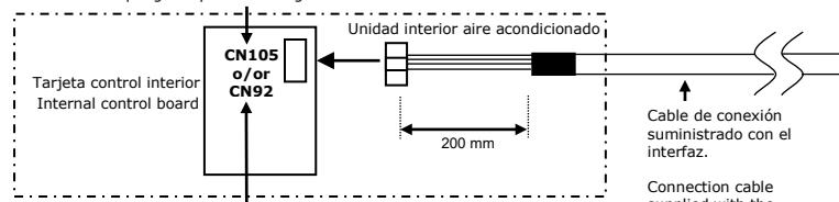
CN105 for Domestic line, CN92 for Mr. Slim line. Check user manual to identify at which line belongs depending on AC model number.
