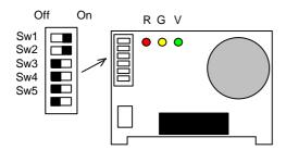
In the standard application EPSTDEMCHA modular chiller addresses for the MicroTech II units:
