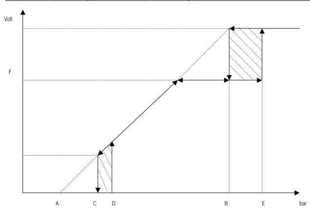
In the case a regulation with cut enabling is not requested, to have a simple continuous fan regulation based on a proportional signal following the condensation pressure set as follows under Manufacturer psw points B,E,F:
