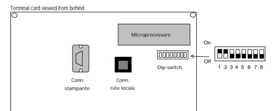
The address of the terminals is set up through the dipswitch bench found on the back. The address is selectable in the 1-16 range by utilising the 1-5 dipswitch. The address value is obtained via the following table (see also previous paragraph):
