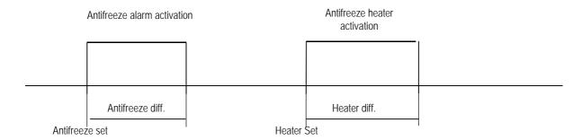
The antifreeze regulation is always energized also when the machine is OFF, both summer working and winter working.
